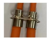
步骤8:将端子部件装入①连接器组件,注意扣盖开槽与壳体上凸起大小相对应。将尾盖推入,完成组装。 Step7:Push parts in step 7 into ①connector component and make sure keyway on ②back cover matches the key on shell。Harness well-finished as the picture shown below
