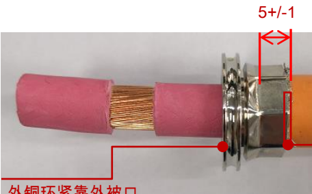
Outer Copper Ring Close to the outer Jacket
